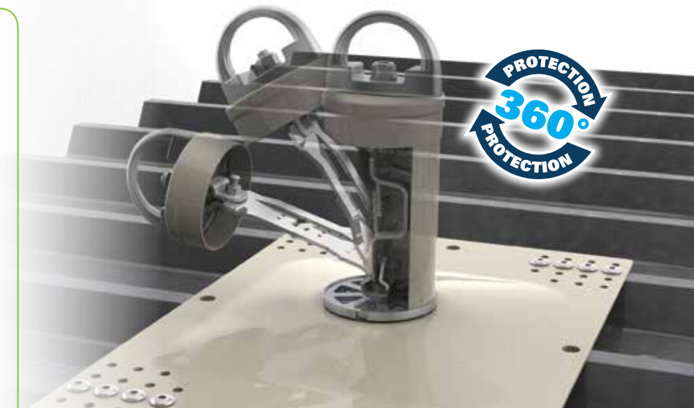
In the event of a fall, the Miller Fusion Roof Anchor Post orients in the direction of the force, the built-in, energy-absorbing component activates and the base remains securely attached to the roof surface.
