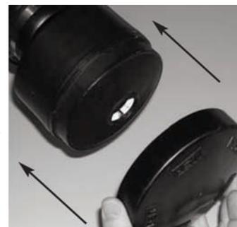
motion for attaching spark cover
