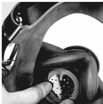
2. Starting at the top, stretch and push the rubber ring of the nosecup under the plastic retainer ring of the speaking diaphragm assembly.
