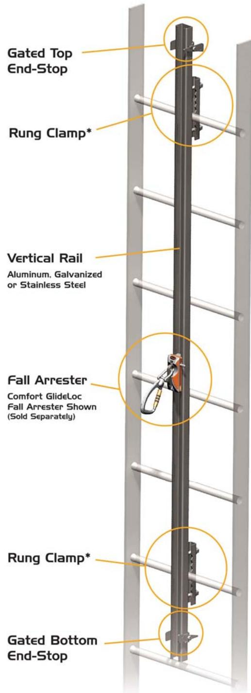
\*Minimum four (4) rung clamps required for each system.
