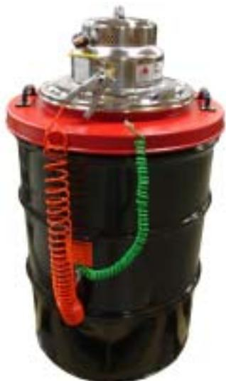
This 55 gallon drum vacuum is supplied complete with a cart, filters, motor, and accessories. Conductive hose is provided and will allow static charge buildup to pass to the recovery can and then to the ground wire. Aluminum tools should only be used and are provided to prevent sparking. The drum head is grounded to the 55 gallon drum. A ground wire and clamp must be attached to a grounded source in order to dissipate static charges.
